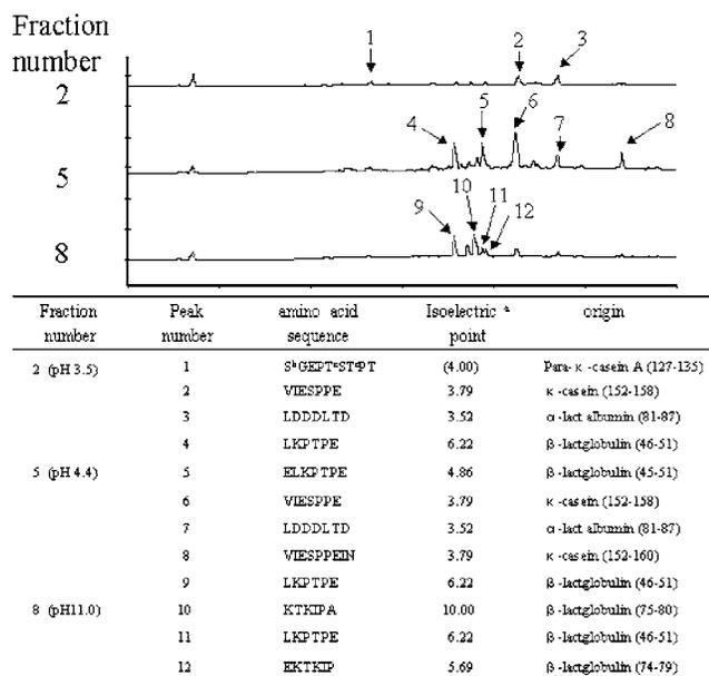
**Figure 10.** Summary of characteristics of isolated peptides from autofocusing fractions of whey protein hydrolysate by method 2. Peptides were isolated by a series of SEC and RP-HPLC. <sup>a</sup>This value was estimated without considering possible modification with phosphate. <sup>b</sup>Potential residue for phosphorylation. <sup>c</sup>Potential residue for modification with o-link sugar chain.
