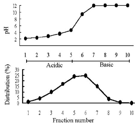
**Figure 5.** pH gradient and distribution of peptide in the autofocusing fractions of casein hydrolysate by method 2 for 24 h.
