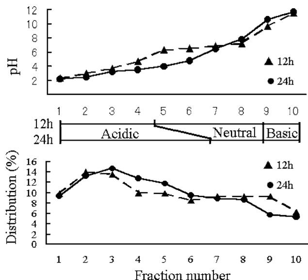
**Figure 3.** pH gradient and distribution of peptide in the autofocusing fractions. Casein hydrolysate was fractionated according to method 1 for 12 and 24 h. See Materials and Methods for details.
