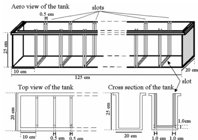
Figure 1. Schematic drawing of a tank for autofocusing.
