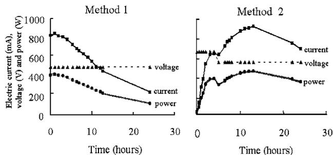
**Figure 11.** Electric current and power developed by autofocusing according to methods 1 and 2. Casein hydrolysate was used as sample.
